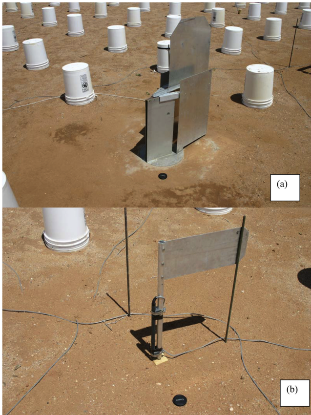
Figure 3. (a) Self-orienting sand trap used to measure saltation flux. A balance is located beneath the wedge-shaped slotted trap that receives the sand moving in saltation. (b) Piezoelectric Safire saltation sensor attached to a self-orienting vane.
